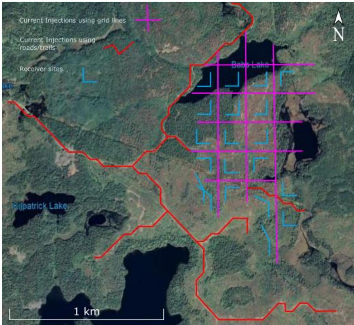
Figure 2: Satellite Image Gowganda East – 3D IP Grid Layout
